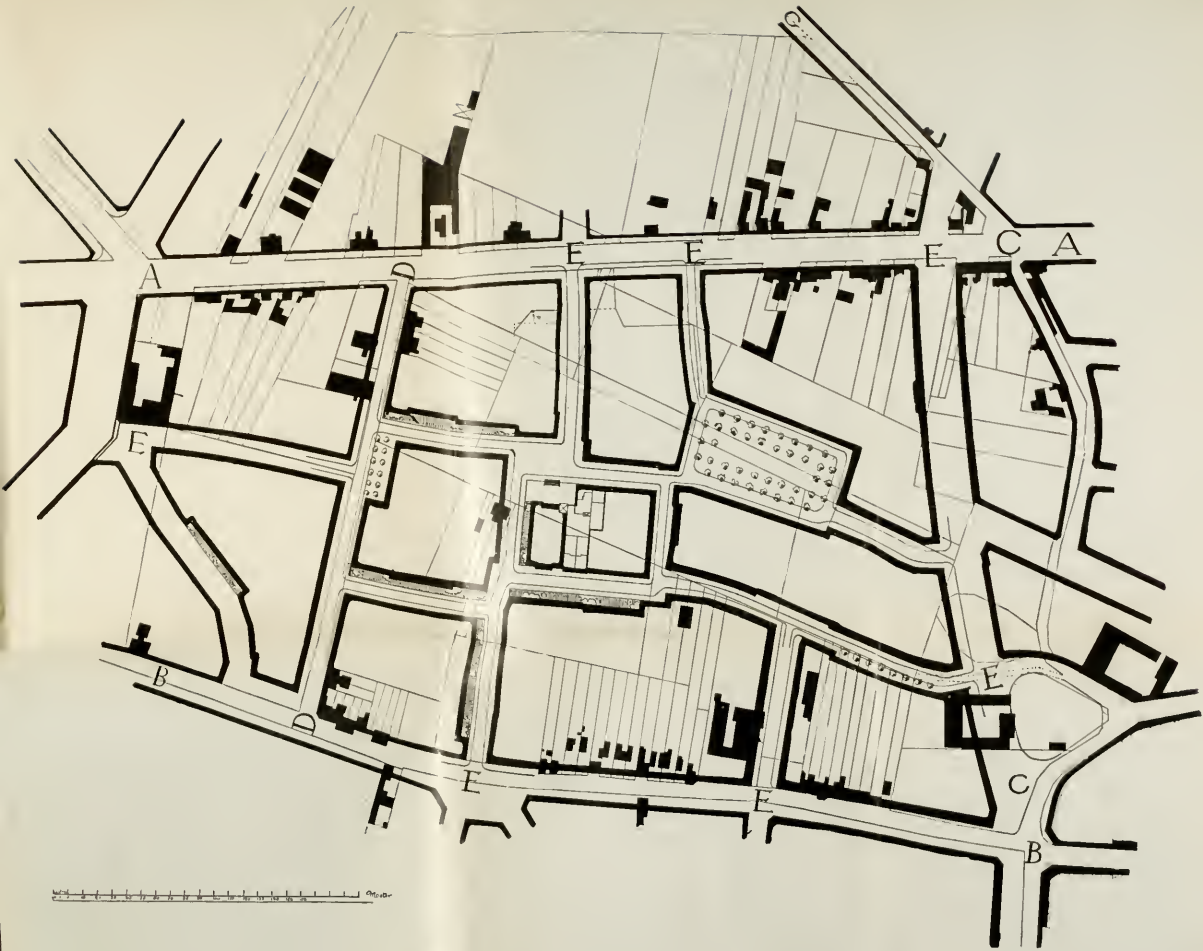
Field Map V - Calicut. An example of the modern street planning as practiced in Calicut. The roads AA and BB were laid out and made at an earlier period. The roads CC, DD, and EE are the newer roads for delineating the areas between the main roads. CC and DD follow approximately existing tracks. The heavy line is the building line. It is interesting to note, along the road AA, the difficulty that has arisen in placing the buildings owing to the mass of encroachments of the old property boundaries, which are not square with the street.
